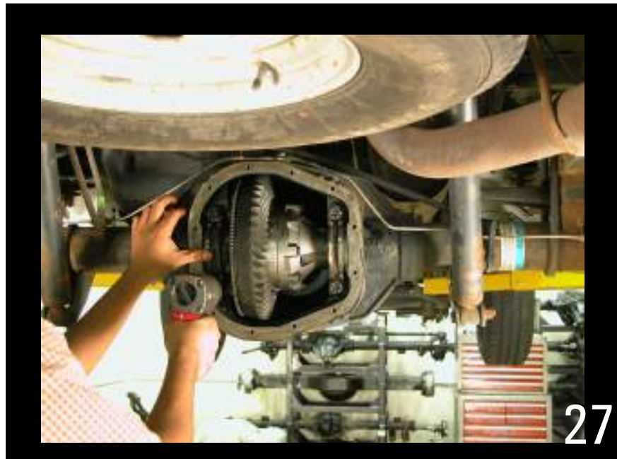
Put bolts in with impact wrench to make sure differential is seated properly in journals.
