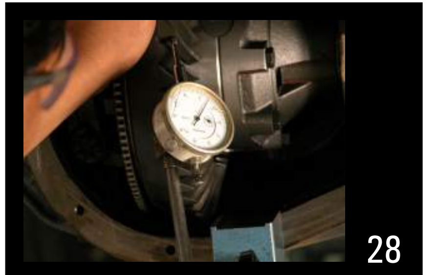
Check backlash. If it is different from that previously measured (picture 3) differential shims will need to be changed in order to re-establish the original backlash measurement. The differential must fit snug into the housing. A total of .006" (.003" per side) of bearing preload is required for proper bearing seating.
