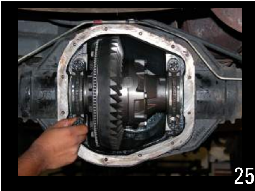
Reinstall bearing caps.
