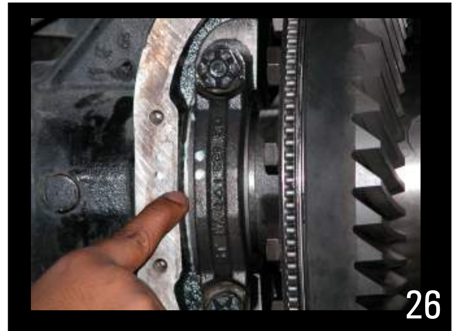
Note the marks you made on the housing and bearing caps to ensure caps are installed on the correct side.
