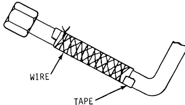
7. Wrap an additional coating of tape over the wire.
