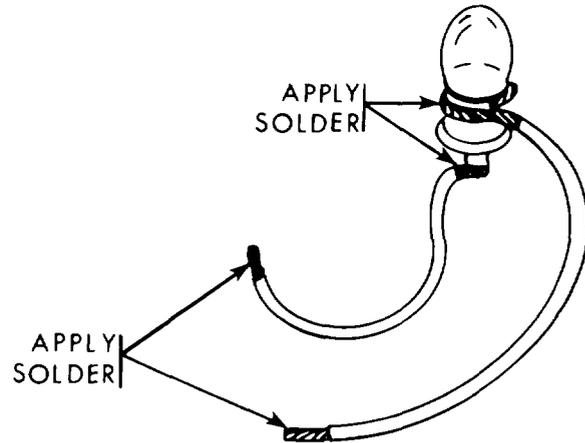
2. Making an ohmmeter (continuity tester).
