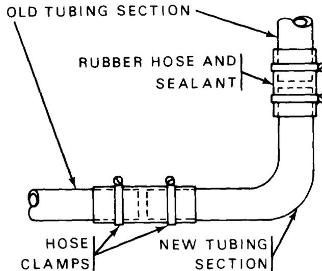
7. Record the BDAR action taken. When the mission is completed, as soon as practicable, repair using standard maintenance procedures.
