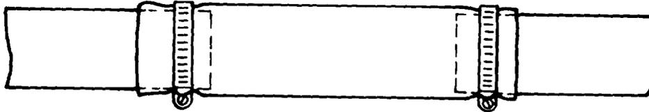
4. Slip the hose over the ends of the damaged hose.
