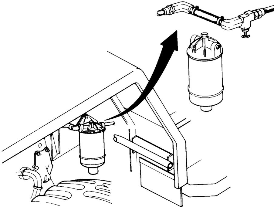
3. If a coupling is not available, cut the fittings off the fuel lines.
