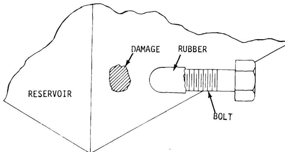
3. Insert slivers of wood if necessary to help ensure a better seal.
