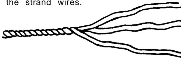
5. Trim the wires to make a tapered end for wrapping the wires tight against the rope body with seizing strand, or wrap with copper wire or friction tape to safety-cover the exposed wire.
