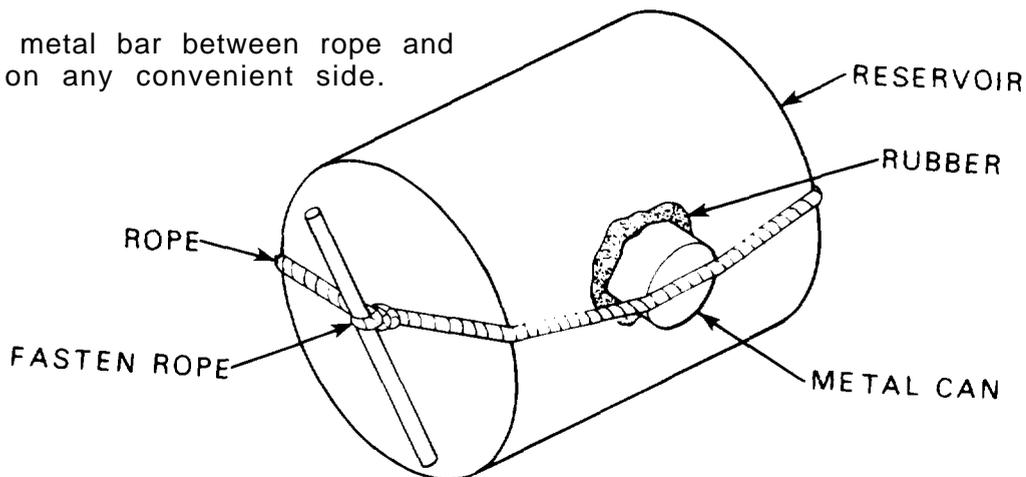
7. Twist metal bar to tighten rope until fluid stops leaking.
