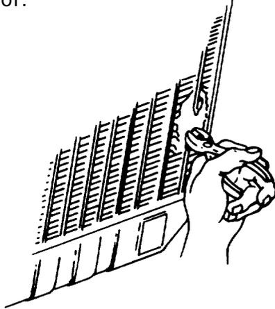
2. Inspect the radiator to pinpoint the leak.
