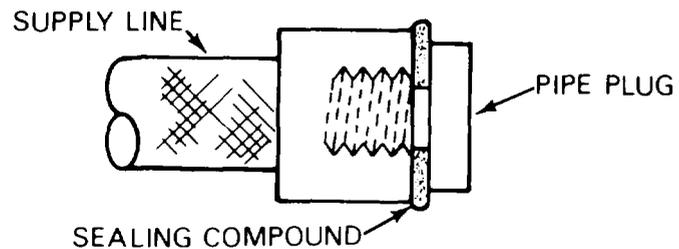
Option 3: High-Pressure Line Repair with a Cap.
