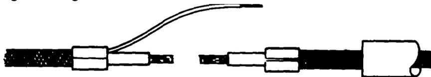
4. Install a grounding sheath connector to the other side of the break. Do not crimp this one yet.
