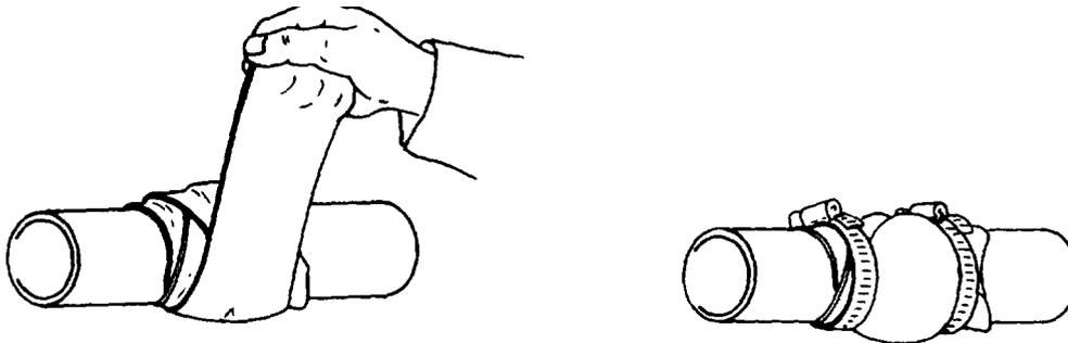
4. Wrap the inner tube as tightly as possible on the hose.
