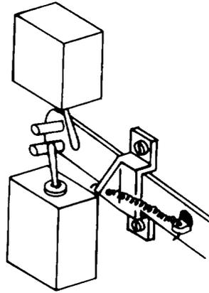
13. Turn the POWER switch to LOW position. Both of the circuit breaker levers should remain in the ON position.
