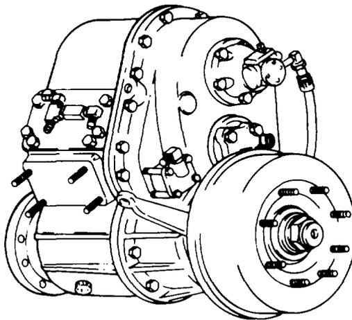
4. Apply sealer around peg to ensure secure seal.
