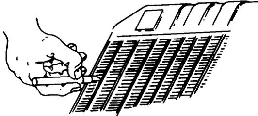
2. Inspect the radiator and pinpoint the leak.
