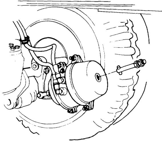
1. Use a caging bolt tool and turn in a direction that will retract the pushrod and compress the power spring in the brake chamber.
