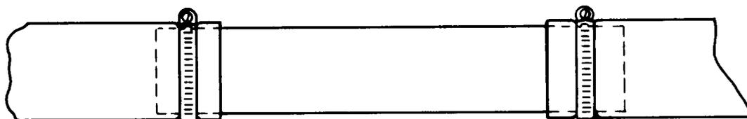
4. Insert the pipe into the damaged hose ends.
