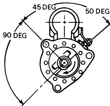
FIGURE 8-1-B. Pinion housing position for LD-465-1 and LD-465-1C, and LDT-465-1C engine applications.
