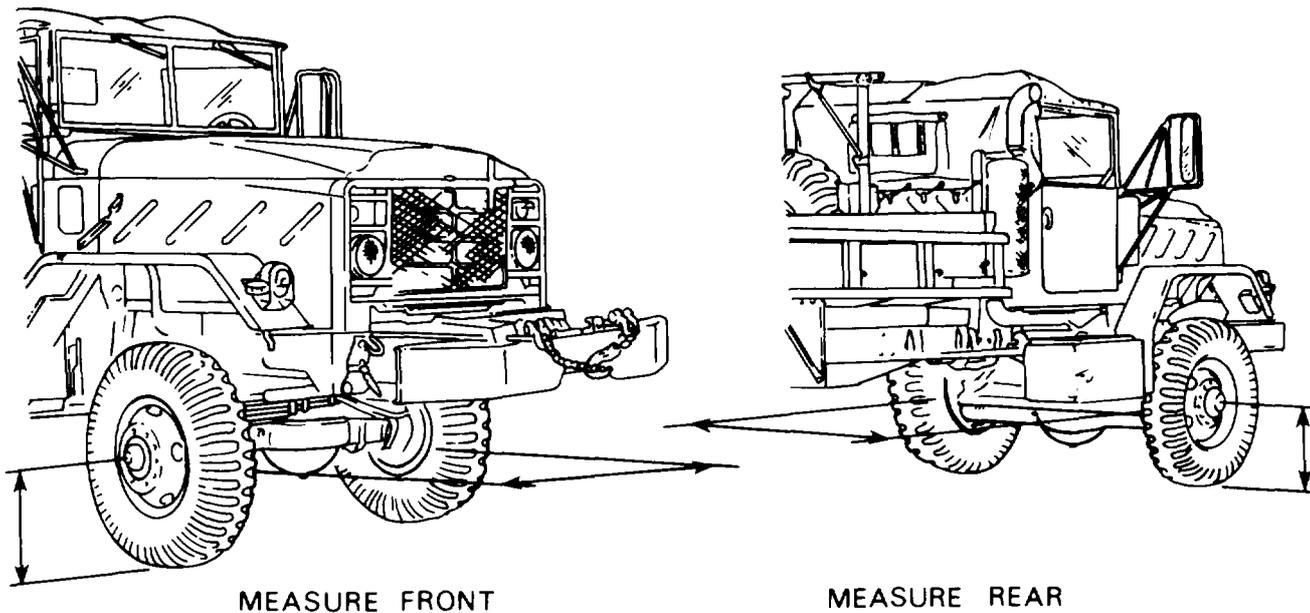
d. Measure and record distance between marks. The front measurement should be 1/4 inch shorter than the rear.
