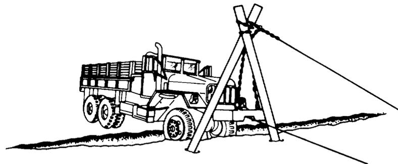
2. Lash the poles together at the top with a figure-eight or girth hitch as shown below.
