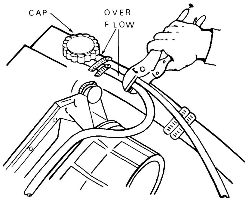
7. Plug overflow lines on surge tank coolant systems if so equipped.
