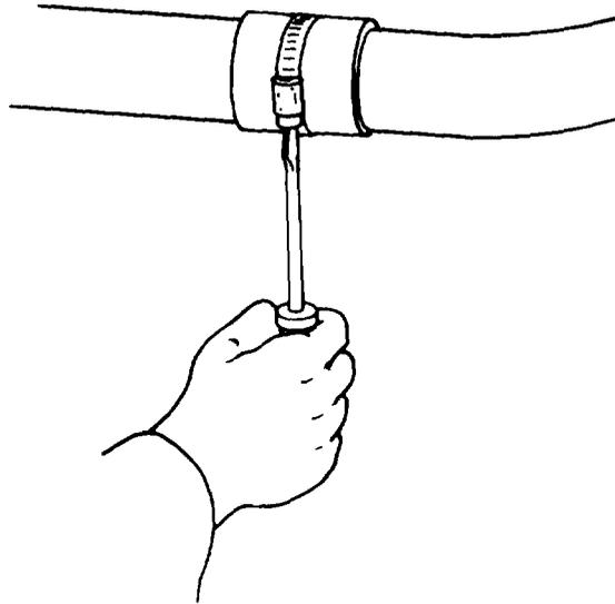
4. Wrap a nonporous material (raincoat, rubber mat) over the leak.
