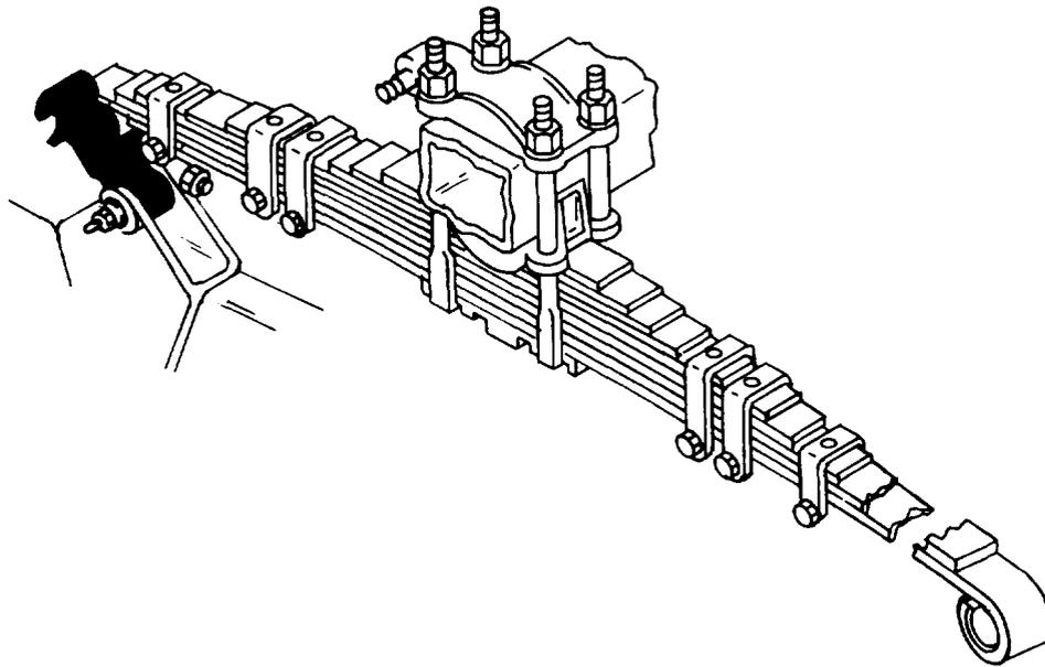
4. Weld the broken leaf springs with 1/4-inch passes. Allow each pass to cool. Keep alternating the welding process until all broken springs are welded.
