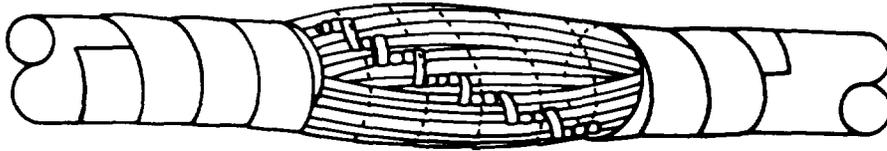
5. Stagger splices, when possible, at least one splice length.
