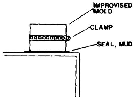
6. Melt approximately 6 oz of lead or solder in a metal can or cup and pour it into the improvised mold.
