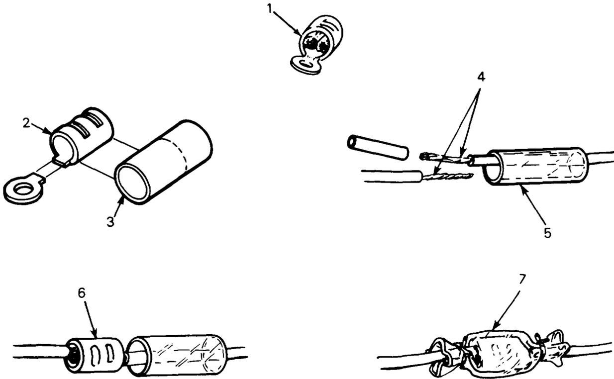
3. Cut insulating sleeve 1 inch longer than the barrel.
