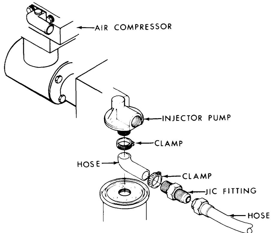
3. Install JIC-to-pipe adapter fitting.
