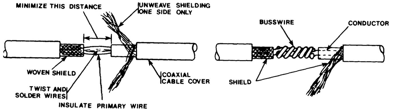
6. Lay the unwoven shielding over the insulated splice and make contact with the woven shield on the other side. Distribute the unwoven shielding carefully around the diameter of the wire and solder or wrap with busswire.
