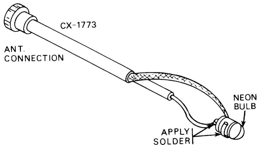
a. An RF transmitter output tester can be made from a neon light bulb and a piece of CG-1773 RF cable. Solder the bulb to the cable as shown in the illustration. Connect the cable to the ANT connection on the front of the radio. When the radio is keyed, the bulb will glow if RF power is present at the antenna connection (this does not verify transmitter frequency accuracy).
