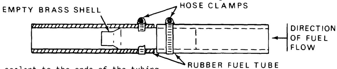
3. Apply sealant to the ends of the tubing.
