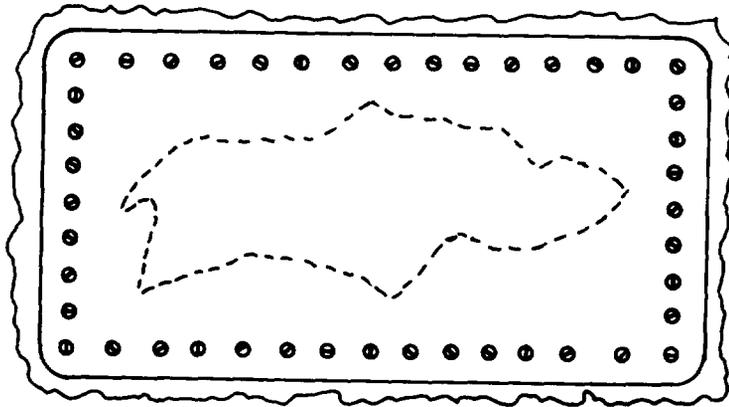
6. Drill holes in plate and tank approximately 1 inch apart. Apply sealer to the patch and rivet or screw the plate to the fuel tank.
