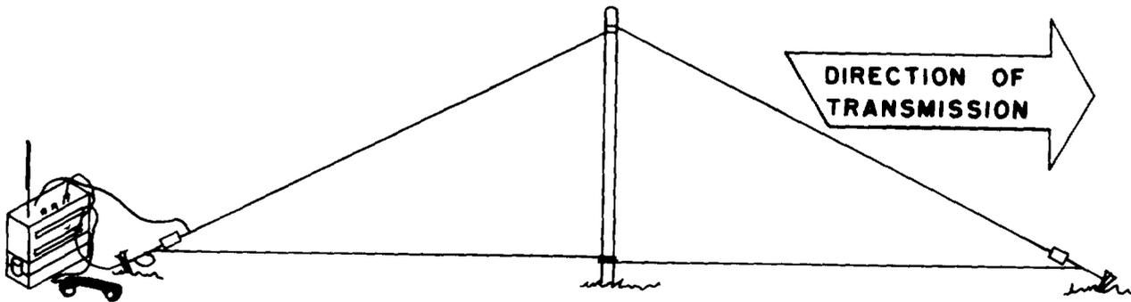
3. Move your vehicle approximately 50 feet from the support. Keep the support in line with and between you and the desired station.
