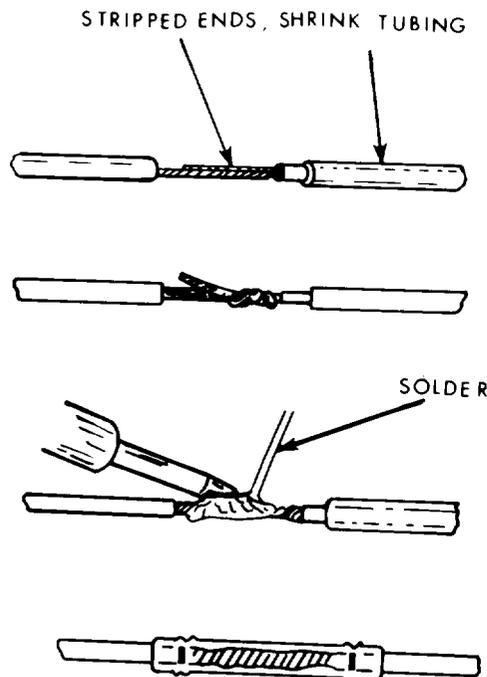
3. Lay the stripped ends side by side.
