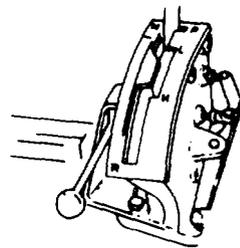
2. Clamp vise grips onto the remaining portion of the shift lever.
