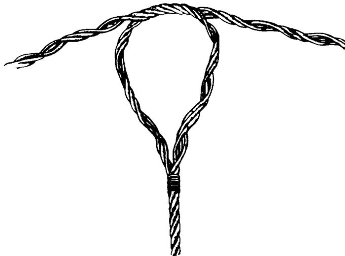
3. Start laying the strand sections alternately back into the rope grooves, continuing until sections are laid as deep into the throat as possible, allowing the six strands and core to project past the throat of the loop.
