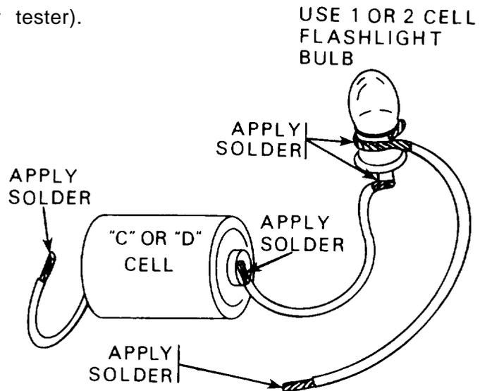
3. Making an RF Transmitter Output Tester.
