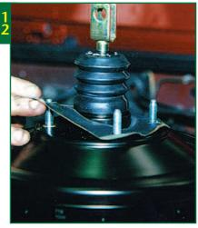
You will need to refit the old gasket to the new servo; a replacement gasket is not supplied with it
