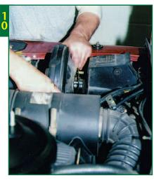
Carefully pull the servo unit away from the pedal box assembly so as not to damage the sealing gasket
