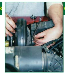
Next remove the four nuts at the back of the servo unit that secure it to the pedal box; accessibility isn't bad
