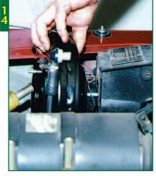
The new servo unit can be fitted to the pedal box assembly, but don't bolt it up yet, to allow for movement
