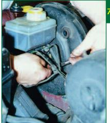
Next step is to undo the two nuts that secure the brake master cylinder to the servo unit itself
