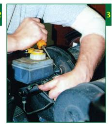
Using a screwdriver, carefully prise out the plastic connector for the vacuum supply hose from the servo unit
