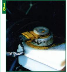
Finally re-fit the vacuum hose and electrical lead (shown) and check that the brake pipes are not rubbing on each other.
