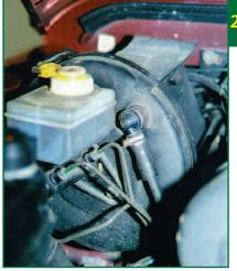
Disconnect the electrical supply lead for the low fluid-level warning light from the top of the brake fluid reservoir
