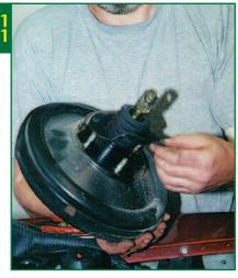
With the servo now free from the pedal box, carefully remove the rubber gasket from the four retaining bolts
