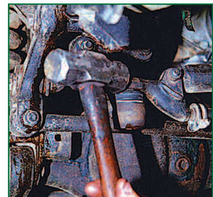
Use a hammer to 'split' the ball joint, as you are going to reuse it. A fork splitter may damage the rubber boot
