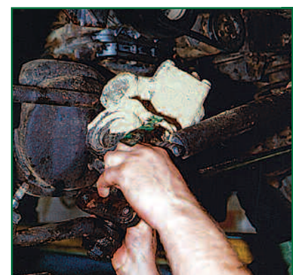
The box does take a bit of manoeuvring out; you might find it easier if you remove the steering damper
