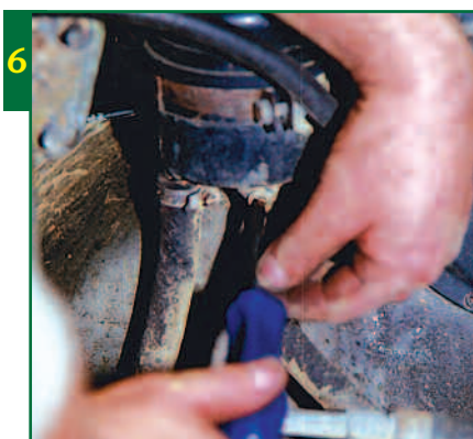
On the 200 Tdi Defender, you will need to undo the return pipe between the reservoir and the steering box
