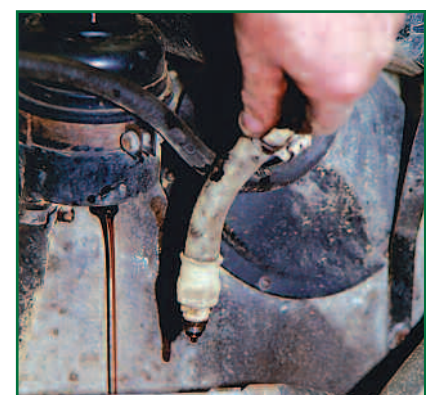
Now free from the reservoir, the return pipe can be unscrewed from the top of the power steering box
