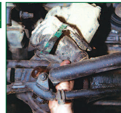
Once the bolts have been removed, the power steering box is now free and can be removed from the vehicle
