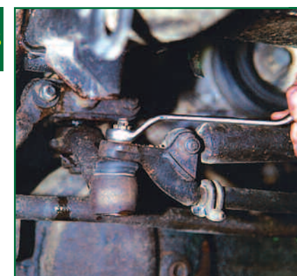
Next remove the split pin from the castle nut which retains the drop arm ball joint, and undo the nut itself
