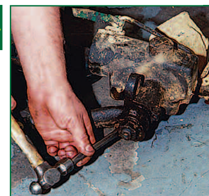
With the steering box on the ground, the tab washer holding the drop arm nut can be opened and the nut removed
