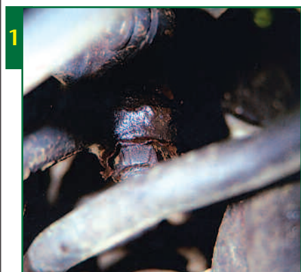
Warning signs: power steering fluid seen leaking from the box, dripping down the sector shaft or drop arm
