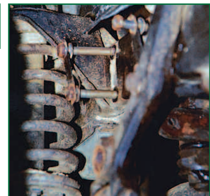
Once the tab plate has been hammered open, the nuts can be undone and the bolts can be pulled out
