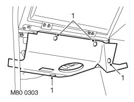
1. Remove 4 studs securing toe board and remove toe board.
