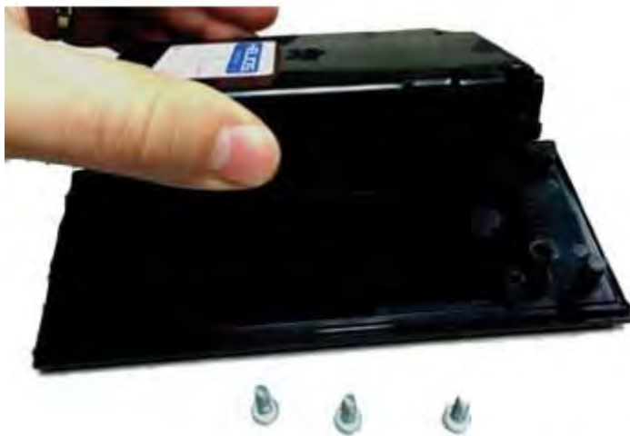
Fig. 26: Lifting Wireless Charging Module From Tray Assembly Courtesy of CHRYSLER GROUP, LLC
