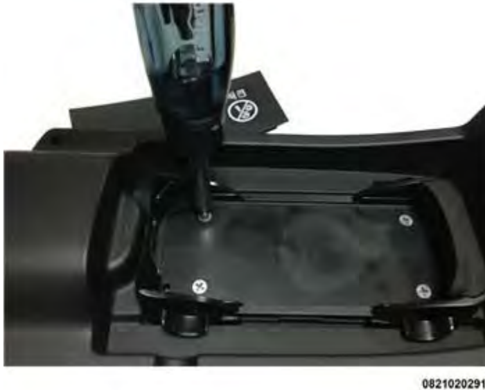
Fig. 21: Removing Screws Using A Phillips #2 Screwdriver Courtesy of CHRYSLER GROUP, LLC
