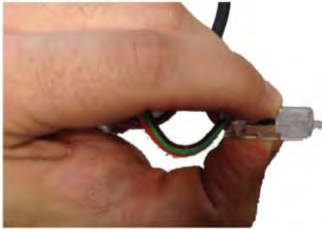
Fig. 35: Squeezing LED Lens Retaining Clips Courtesy of CHRYSLER GROUP, LLC
