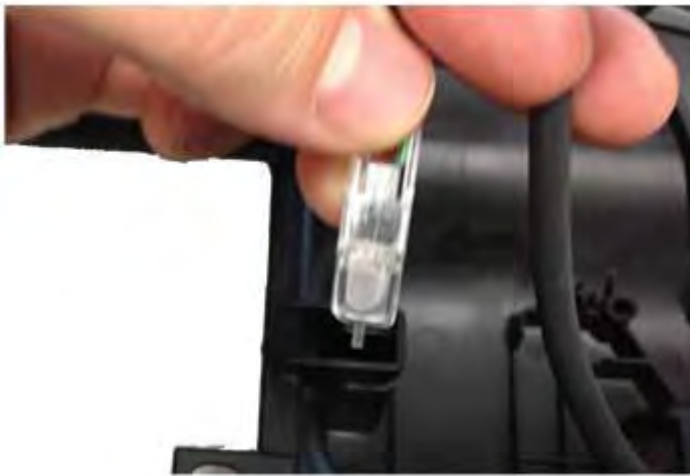
Fig. 36: Inserting LED Lens Into Lower Tray Courtesy of CHRYSLER GROUP, LLC
