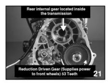
The view of the extension case area is similar to the current 4EAT Phase 2. The difference is the Reduction Drive Assembly.
