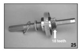
A Sun Gear made on to the end of the Rear Drive Shaft receives the power and transfers the power to the shaft.
