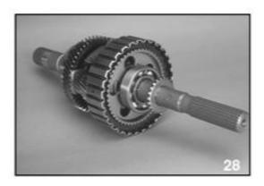
The TCM adjusts the duty ratio of the MPT clutch to maintain the optimum transfer of power. A large speed difference in the rear to the front wheels results in the MPT clutch locking the Rear Drive Shaft to the carrier.
