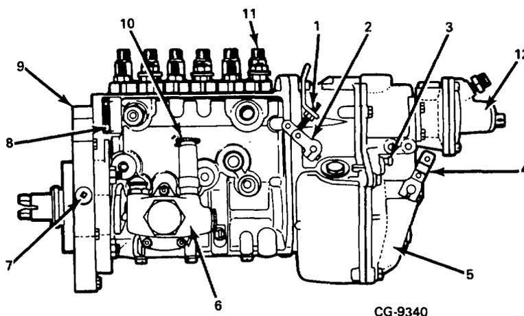
Figure 1. Robert Bosch Model MW Fuel Injection Pump
