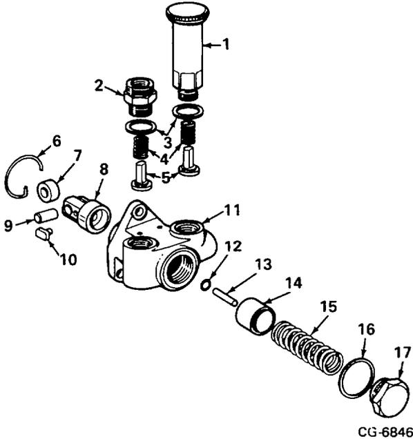
Figure 33. Exploded View of Fuel Supply Pump
