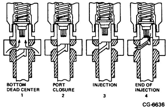
Figure 3. Four Principle Plunger Positions of Injection Cycle
