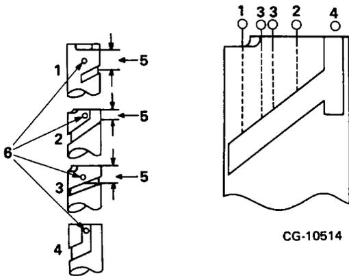
Figure 5. Helix and Charging Port Metering Positions
