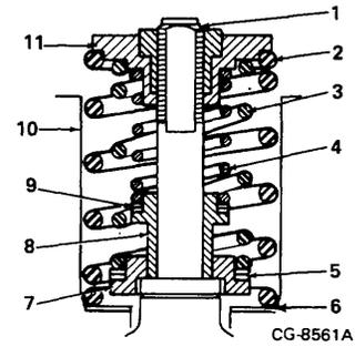
Figure 4. Sectional View of Flyweight Spring Installation
