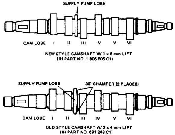
Figure 6. Camshaft Identification
