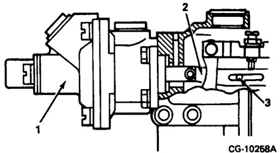
Figure 8. Removing Aneroid
