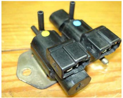
Electronic signals from the transfer box, to the gearbox ECU govern the operation of solenoids that control the vacuum feed to open and close the actuator located on the front differential.
