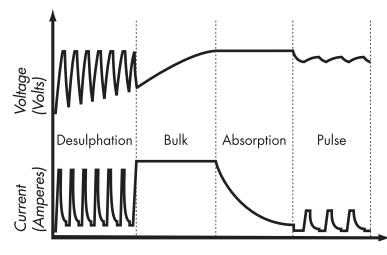
**Desulphation** – Desulphation with pulsing for sulphated batteries.
