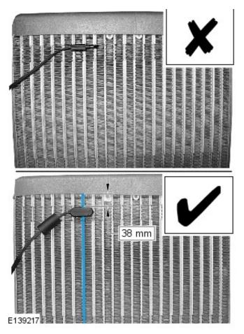
Install a new HVAC evaporator temperature sensor.
