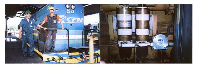
The locomotive used was an ALCO RSD8 with a 1050hp engine. 8 different load points were measured for 10 minutes each, first without and then with and LG-X 1500 Fuel Conditioner installed.
